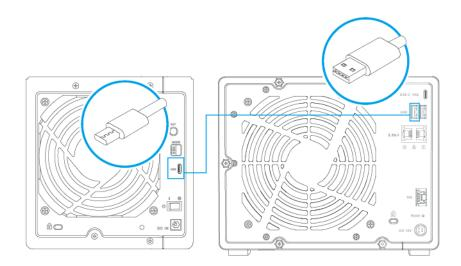
Connecting to a USB 3.2 Gen 2 Type-A port on the NAS.
