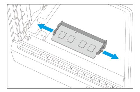
**b.** Verify that the module has tilted upward and is completely released from the slot.
