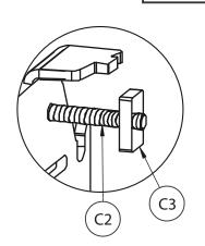
ii. Slide item C1 down the front slots of item A1 to the correct height and tighten items C2.
