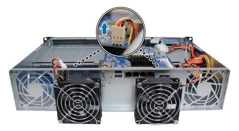
**b** Remove the screws that secure the fan guard from the malfunctioning fan.
