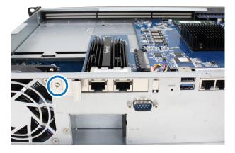
Note: Confirm that the connector is fully inserted. Otherwise, the network interface card might not be able to function properly.
