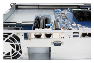
c Place back the latch and fasten the screw that you removed in step 2-a to secure the newly inserted card in
