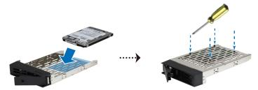
3 Insert the loaded drive tray into the empty drive bay.
