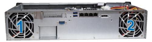
3 Loosen the screws that secure the fan to the back cover as shown below.
