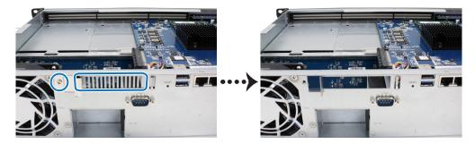
**b** Align the card's connector with the expansion slot and insert the card into the slot.
