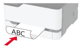
• Load envelope with the flap side down and against the right side of the paper guide.
