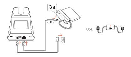
• Connect one end of the telephone interface cable to the back of the base
