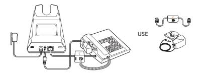
**IMPORTANT** *Cisco* phones use configuration **D** on the bottom of the base. Most other phones use the default configuration **A**.
