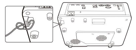
**NOTE:** The security slot can also be used as a safety anchor if the projector is mounted to the ceiling.
