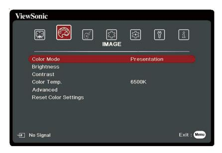
3. Press ▲/▼ to select the menu option. Then press Enter to display its sub-menu, or press ◀/▶ to adjust/select the setting.
