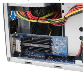
**Note:** Make sure the connectors are fully inserted. Otherwise, the network interface card might not be able to function properly.
