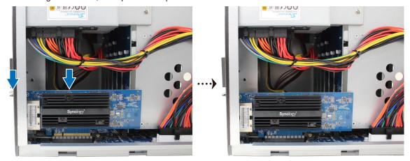
c Push back the clip to secure the newly inserted card.
