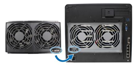
**b** Make sure that all 6 push pins on the new module are pulled outwards before the module is placed into your Synology NAS, and then press the push pins back into place to secure the fan module.
