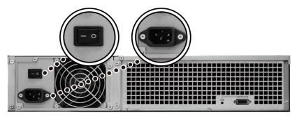
**b** For RX1217RP, connect one end of both power cords to a power port on the RX1217RP, and the other to a power outlet.
