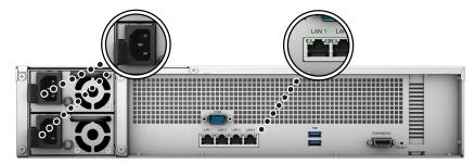
3 Make sure the Power Supply On/Off Switch<sup>1</sup> is turned on ("-").
