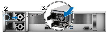
4 Prepare a new PSU. Insert it into the empty slot until you hear a click.
