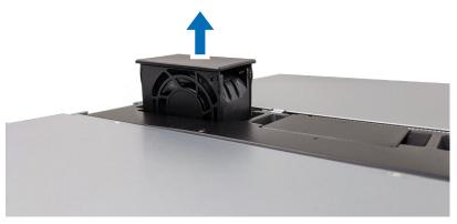
**5** Prepare a new fan and slide it into the the RS2421+/RS2421RP+. Make sure that the fan is aligned properly, as shown below.
