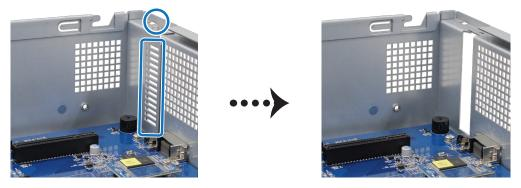
**b** Align the card's connector with the expansion slot and insert the card into the slot.
