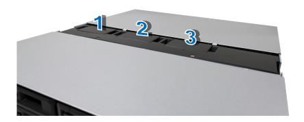
4 Find the malfunctioning fan. Lift up the fan to remove it.
