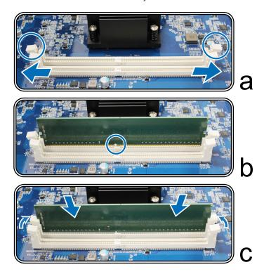
Note: Hold the memory module by its edges and avoid touching the gold connectors.
