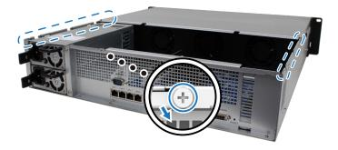
**b** Put back and fasten the screw you removed in step 2.
