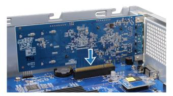
c Fasten the screw that you removed in step 2-a to secure the newly inserted card in place.
