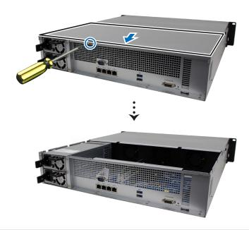
**Note:** When you remove the top cover, sensitive internal components are exposed. Avoid touching anything other than the memory assembly when removing or adding memory.
