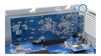
**Note:** Confirm that the connector is fully inserted. Otherwise, the network interface card might not be able to function properly.
