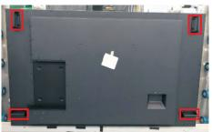
Remove the handles and rear cover, then use a screwdriver to remove 7pcs screws for releasing the PC box.(Torque: 4.5±0.3kgf)
