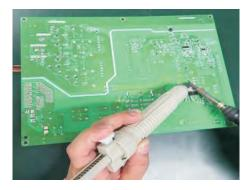
S25-5 Lift the bulk cap. up and away from the PCB.
