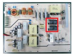
S25-1 Cut the glue between bulk cap. and PCB with a knife.
