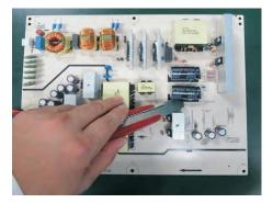
S25-2 Ensure cutting path within the glue, don't touch bulk cap. or PCB.
