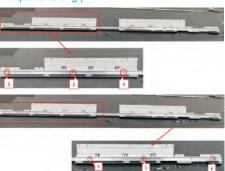
Remove all the bezel and strips and put them on a protective cushion. Open the IR board cover, then use a screwdriver to remove 2pcs screws for unlocking the IR board and holder with front bezel, then use a screwdriver to remove 2pcs screws for unlocking the light pipe with front bezel.
