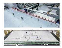
Tear off 2pcs shading mylar tape for releasing the wire hole of the lighter bar. Turn over the panel module with the bracket for screen faced up. Use a thin film(such as Prism film) to disassemble the O/C with glass carefully, then remove the O/C with glass and put then on a protective cushion.
