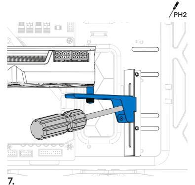
Place the Support Bracket in the Torrent case and insert 2 x Thumbscrew (6-32)
