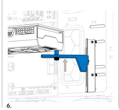
Lock the Support Arm loosely in place with a Screw (6-32)
