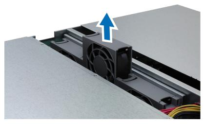
**5** Prepare a new fan and slide it into the the RS2821RP+. Make sure that the fan is aligned properly, as shown below.
