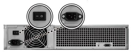
**b** For RX1217RP, connect one end of both power cords to a power port on the RX1217RP, and the other to a power outlet.
