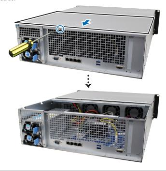
**Note:** When you remove the rear top cover, sensitive internal components are exposed. Avoid touching anything other than the memory assembly when removing or adding memory.
