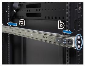
2 Extend the inner rail from the assembly and pull it out.
