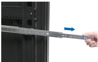
**3** Align the fixing holes of the inner rail to the attachment points on the side of the chassis. Slide the inner rail away from the front panel to attach it to the chassis.
