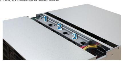
4 Find the malfunctioning fan. Lift up the fan to remove it.
