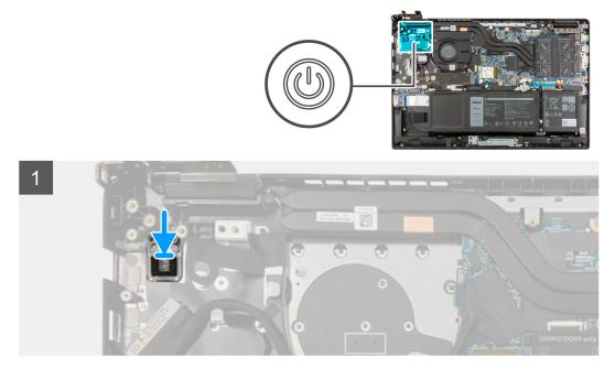
Align and place the power button into the slot on the palmrest assembly.
