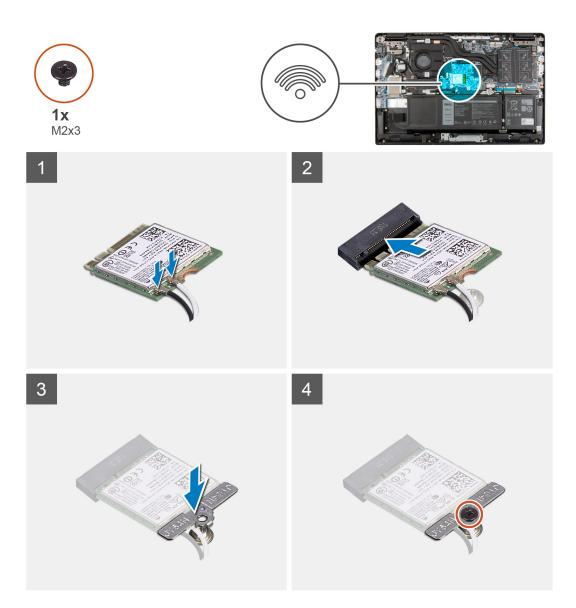
1. Connect the two antenna cables to the connectors on the WLAN card.
