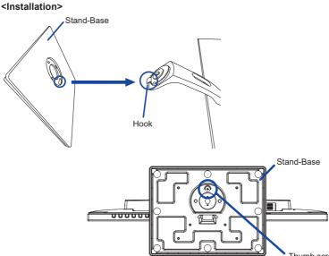
Thumb screw for Stand-Base fixing
