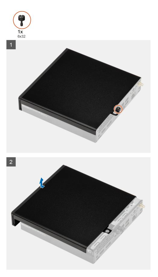
1. Loosen the thumbscrew (6x32) that secures the side cover to the system.
