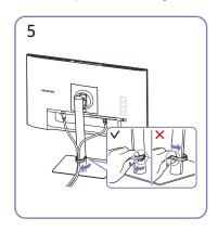
Pull the right side of the HOLDER-STAND CABLE to remove from the stand. The left side of the HOLDER-STAND CABLE can be damaged when pulled forcibly.
