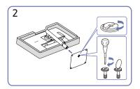
Insert the stand base into the stand in the direction of the arrow. Fasten the screw tightly (using a screwdriver or coin) into the bottom of the stand base.
