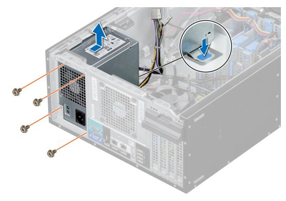
Figure 43. Removing the PSU
