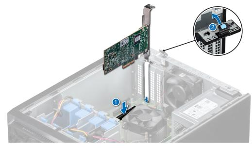
Figure 31. Installing a PCIe expansion card
