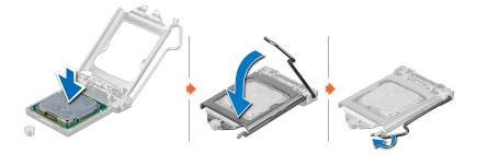
Figure 40. Installing the processor
