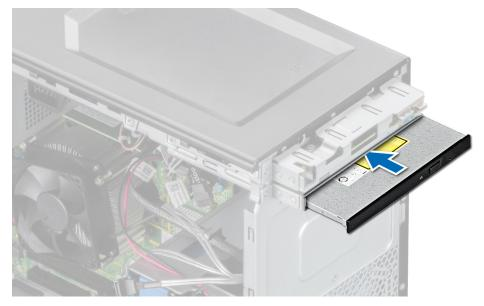
Figure 22. Installing the optical drive
