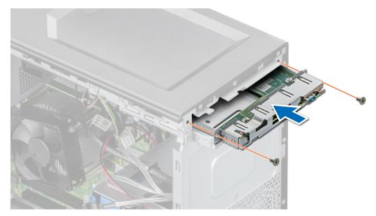
Figure 57. Installing the control panel cage
