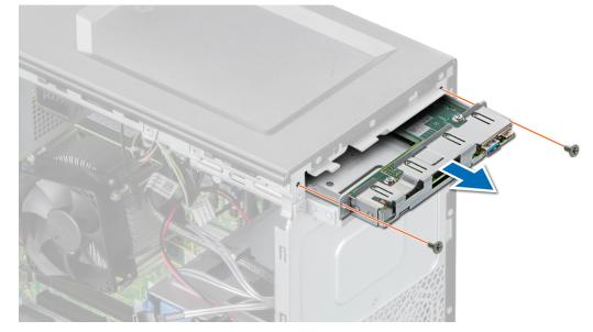
Figure 54. Removing the control panel cage
