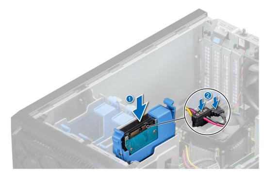
Figure 14. Installing the drive carrier into the drive bay
