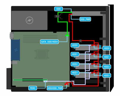
Figure 35. Cable routing - four 3.5-inch cabled SAS drive with storage controller card
