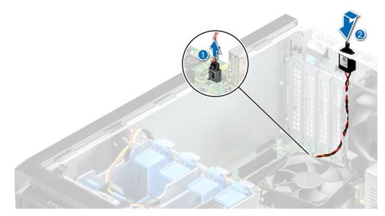
Figure 48. Removing the intrusion switch
