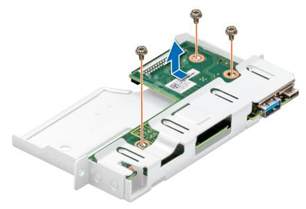
Figure 55. Removing the control panel
