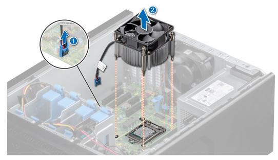
Figure 38. Removing the heat sink
