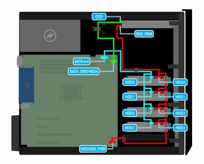
Figure 34. Cable routing - four 3.5-inch cabled SATA drive
