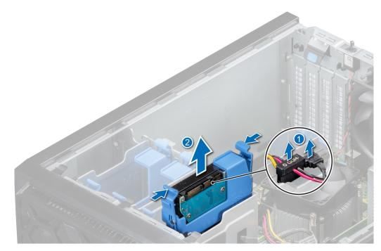
Figure 13. Removing the drive carrier from the drive bay
