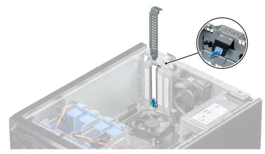
Figure 30. Removing the filler bracket
