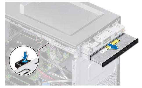
Figure 21. Removing the optical drive
