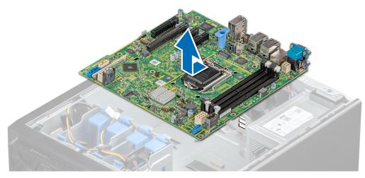
Figure 51. Removing the system board
