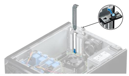
Figure 29. Installing the filler bracket
