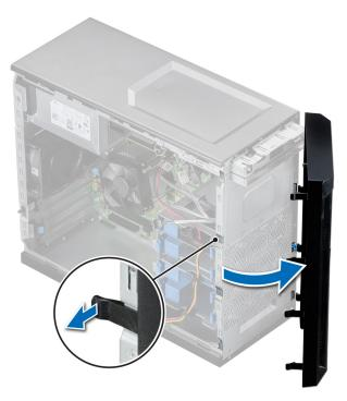
Figure 11. Removing the front bezel
