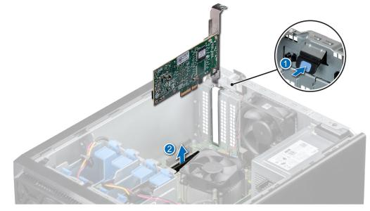
Figure 28. Removing a PCIe expansion card
