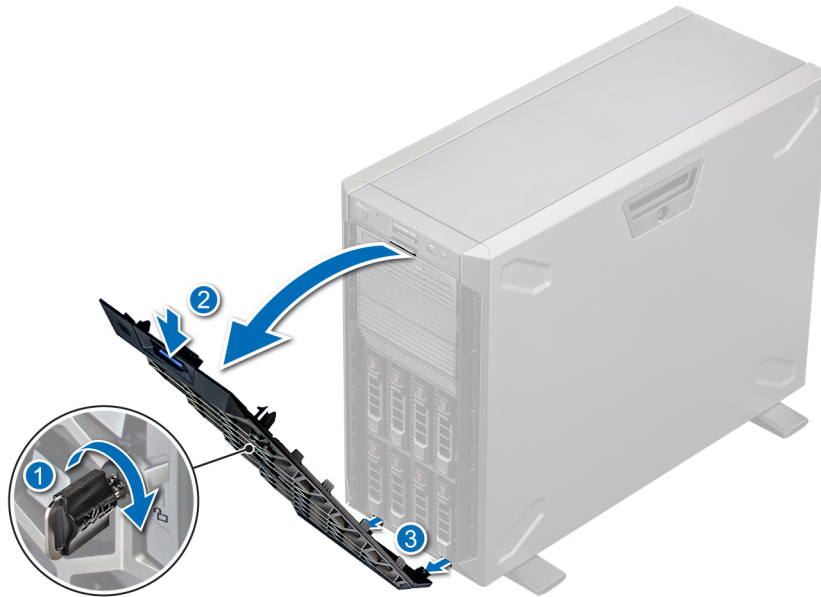
Figure 17. Removing the front bezel
