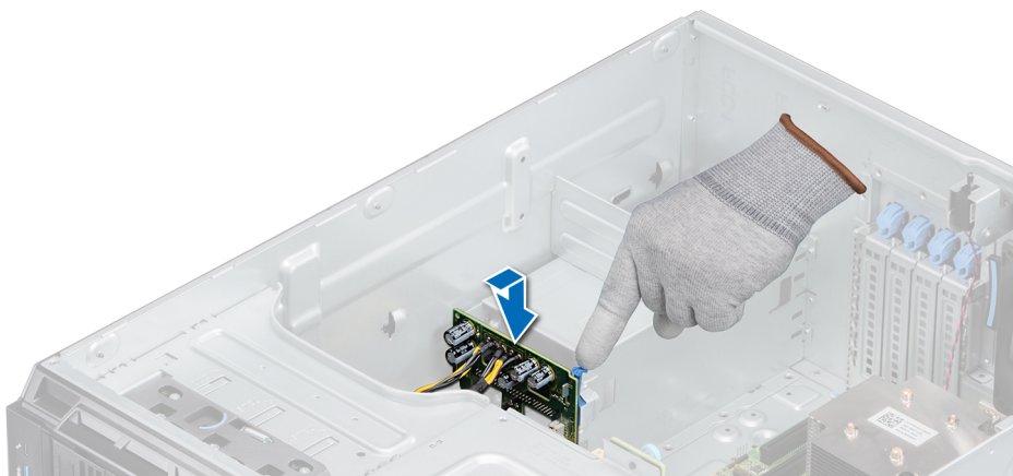
Figure 77. Installing the power interposer board
