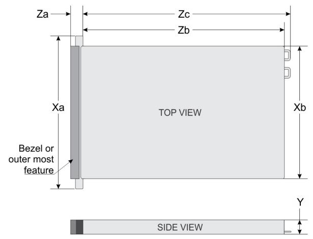
Figure 1. Chassis dimensions
