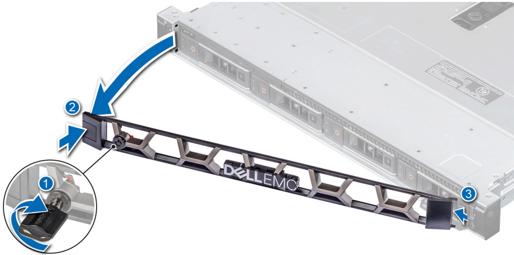
Figure 13. Removing the optional front bezel
