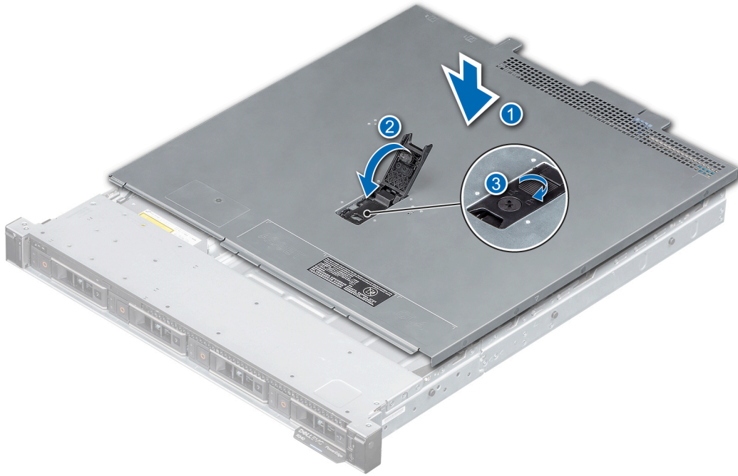
Figure 16. Installing the system cover
