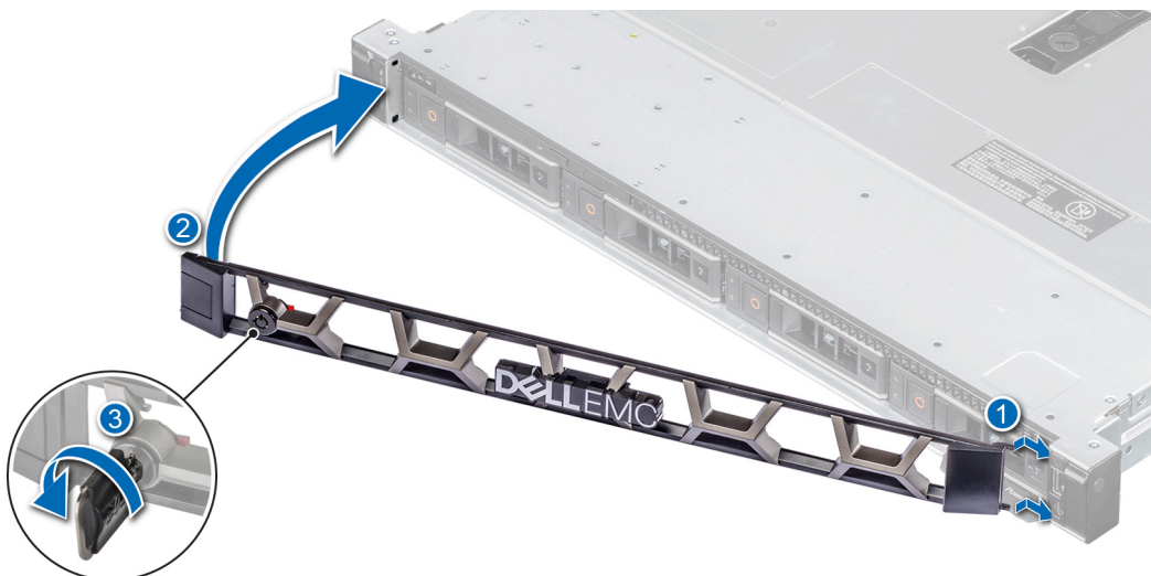
Figure 14. Installing the optional front bezel
