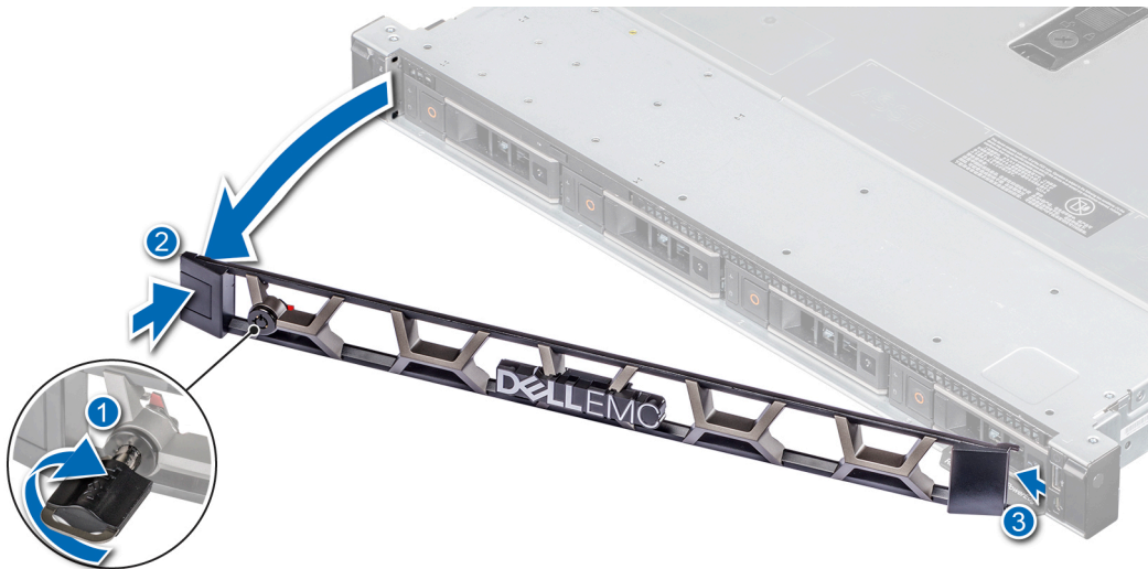
Figure 9. Removing the front bezel
