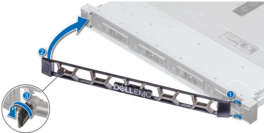
Figure 10. Installing the front bezel
