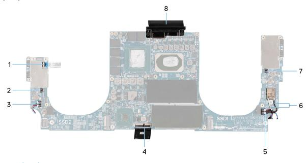
Figure 1. System-board connectors
