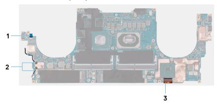
Figure 2. System-board connectors
