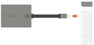
4 Connect a direct HDMI or VGA cable to its respective port on the adapter to output display.
