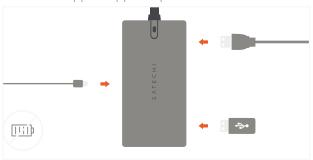
Connect a PD charger to the adapter's USB-C PD charging port.
