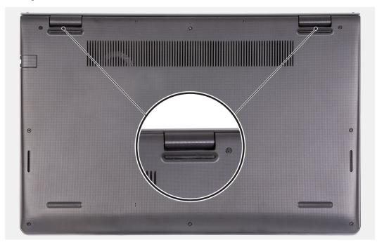
4. Lift and slide the base cover off the palm-rest and keyboard assembly.
