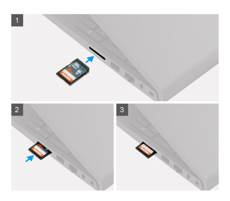
Slide the secure digital into the slot until it clicks into place.
