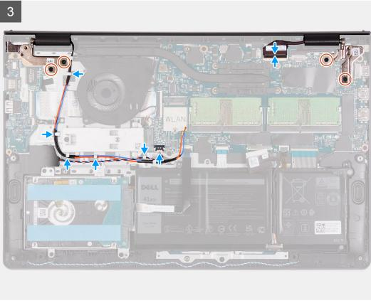
1. Place the display assembly on the system. Align the screw holes on the display hinges with screw holes on the palmrest and keyboard assembly.
