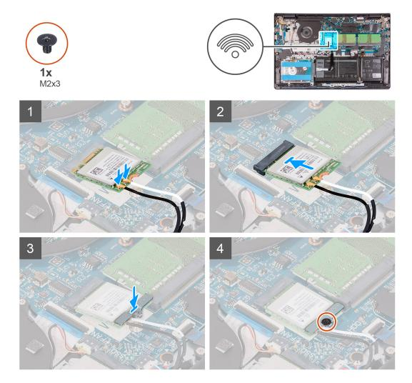
1. Connect the antenna cables to the wireless card.
