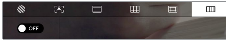
The 'false color' exposure assistance tab
