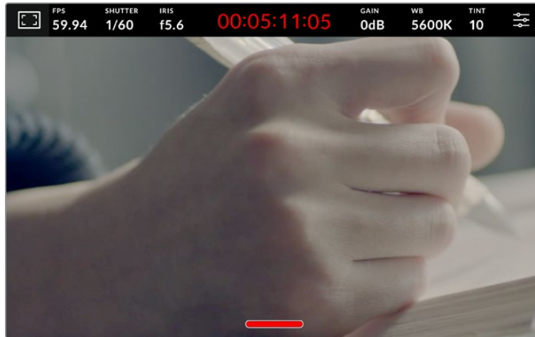
Your studio camera will display a record tally even in clean feed mode
