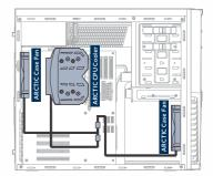
The PST ensures all PWM-controlled devices run at optimized speed (and hence lower noise level) based on actual CPU cooling demand.
