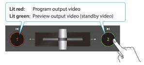
The button you press blinks red, and the video switches. When the video has switched completely, the lit state (red, green) of buttons [1] [2] is exchanged.
