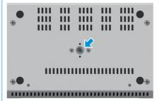
This is used when attaching the V-02HD MK II to a commercially available camera tripod. The socket is threaded for a 1/4" screw.
