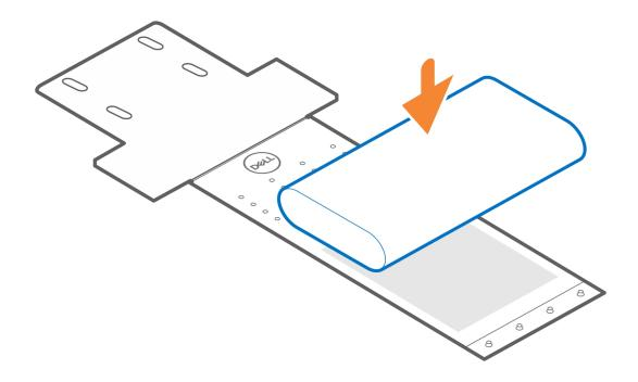
5. Wrap the sleeve around the A/C adapter and insert the retaining tabs into the holes at an appropriate level.
