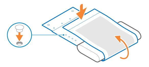
4. (i) NOTE: The screw holes on the A/C adapter sleeve mount are 70 mm (2.756 in.) apart.
