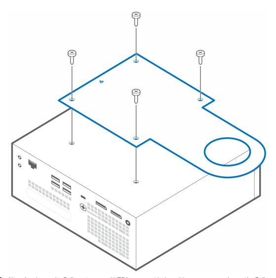
**6.** Align the slot on the Dell monitor stand VESA mount with the cable management slot on the Dell monitor stand.
