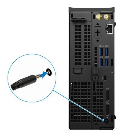
**NOTE:** To conserve battery power, the battery might enter power saving mode. Connect the power adapter and press the power button to turn on the computer.
