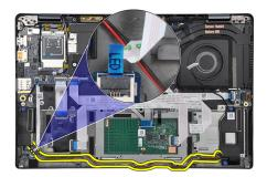
Route the speaker cable underneath the LED board FFC.
