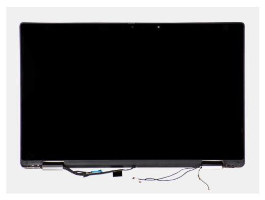
Figure 1. Display assembly with antennae cables
