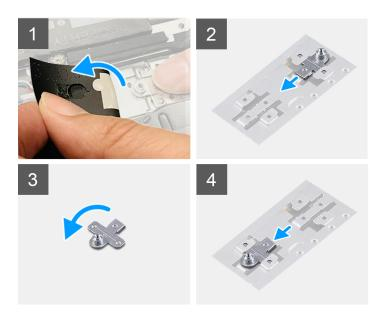
The following image provides a visual representation of the procedure to install the solid-state drive mounting bracket when replacing a M.2 2280 solid-state drive with a M.2 2230 solid-state drive.
