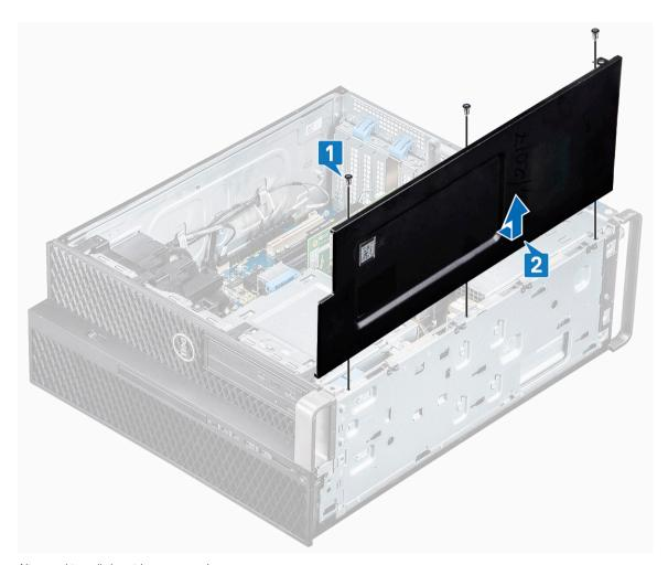
5 Align and install the side cover to the system.
