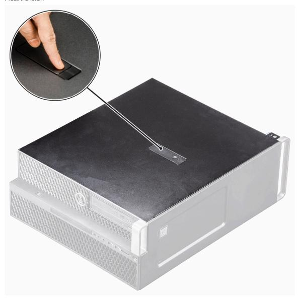
b Pull the latch [1] upward and slide the side cover outwards to remove it from the system [2].
