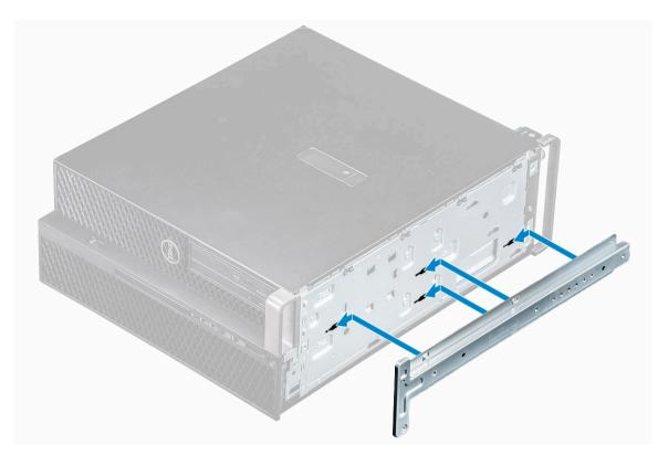
8 Fasten the two (#6-32x1/4) screws to secure the rail on the top of the system chassis.
