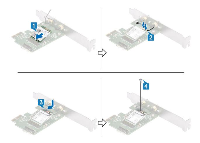
3 Connect one end of the Wi-Fi/BT PCle adapter card cable socket to the connector on the Wi-Fi/BT PCle adapter card.
