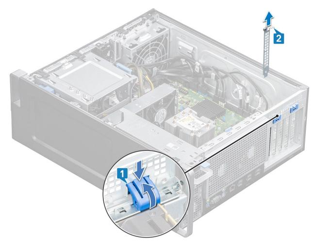
7 Align and place the Wi-Fi/BT PCIe adapter card in the blank PCI filler slot
