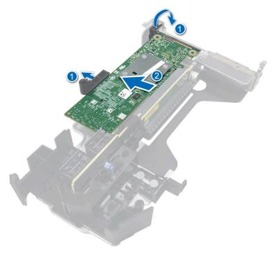
Figure 18. Remove the HBA350i Adapter
