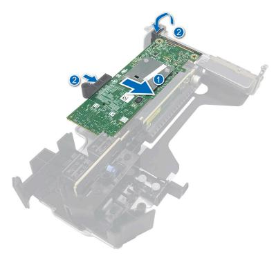
Figure 19. Install the Dell HBA350i Adapter
