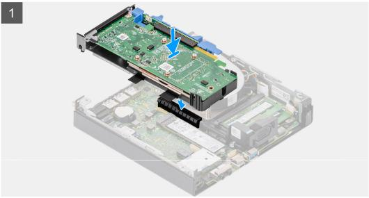
Align the graphics card on the system board and press down firmly. Ensure that the card is firmly seated.
