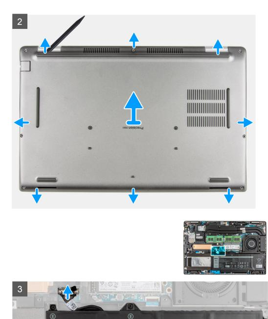
1. Loosen the nine captive screws that secure the base cover to the palm-rest and keyboard assembly.
