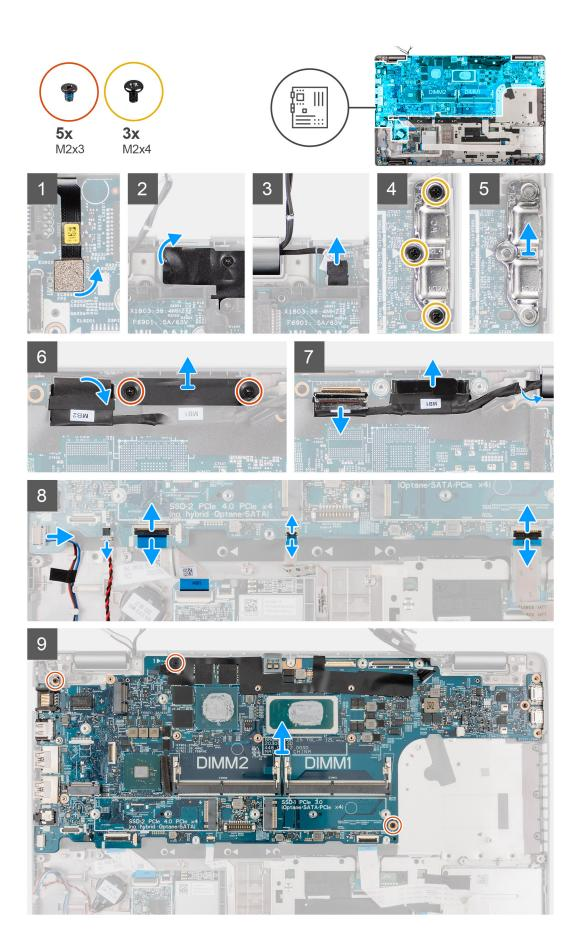
**NOTE:** The system board can be removed and installed with the heat sink attached in order to simplify the procedure and preserve the heat sink between the system board and heat-sink. In order to do so, technicians must also remove the two (M2x5) screws the secure the system fan to the system board.
