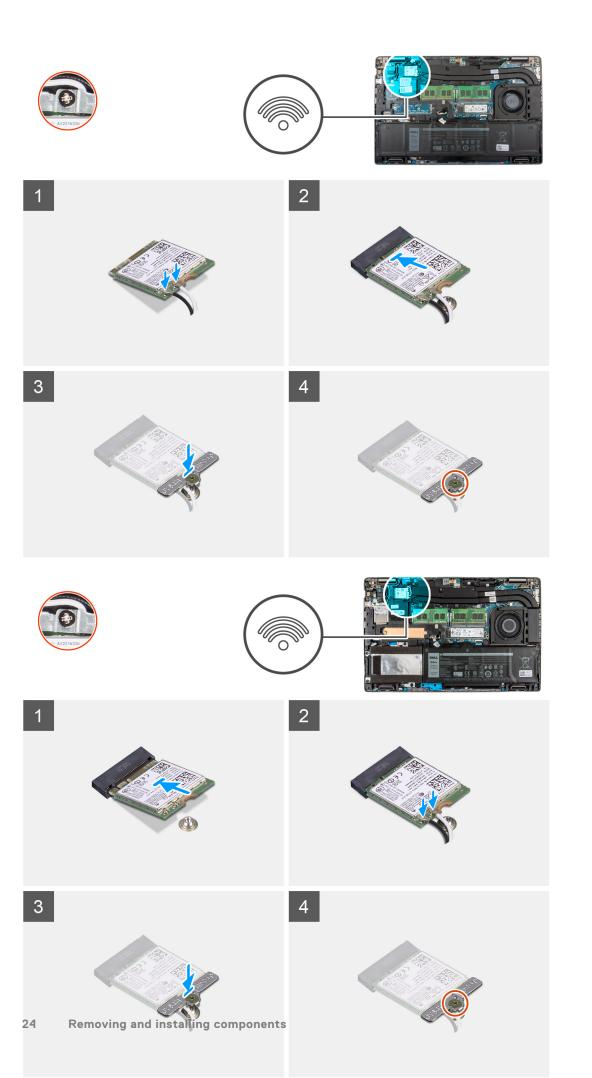
1. Connect the antenna cables to the wireless card.
