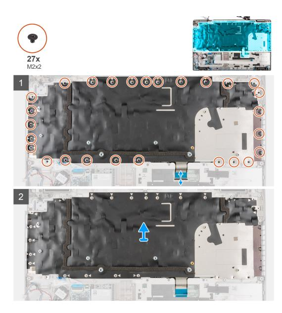
1. (i) NOTE: For models shipped with a USH module, disconnect the USH cable from the keyboard bracket.
