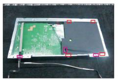
Use a Philips-head screwdriver to remove 8pcs screws for interface board and power board. (No.1 screw size=M4x8, Torque=7±1kgfxcm; No.2~8 screw size=M3x7.5, Torque=7±1kgfxcm)
