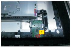
Use a Philips-head screwdriver to remove 18(13+5)pcs screws for unlocking the middle bezel
