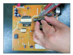
S21-2 Ensure cutting path within the glue, don't touch bulk cap. or PCB.
