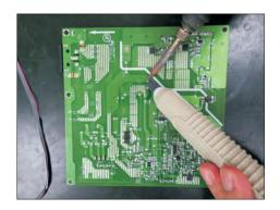
S21-5 Lift the bulk cap. up and away from the PCB.
