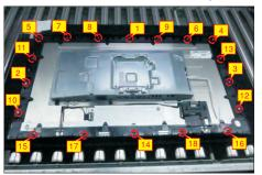
S12 Disconnect the two panel lamp cables from the connectors of the panel. Disconnect the LED cable from the connector of the interface board.
