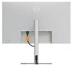
Remove stand from the product.(Press the stand release button, lift the stand up and away from the monitor)
