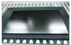
S15 Remove the Mylar tape from the hooks of the bracket chassis module.
