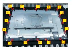
Tear off the tape on the back of panel module for releasing the LED cable, then lift up and take away the middle bezel, and put it on a cushion foam, and then tear off the mylar tape for releasing the LED board.
