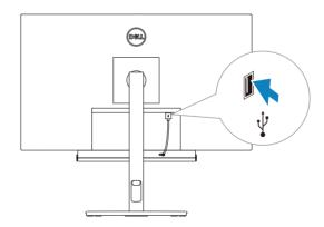
NOTE: For computers that use HDMI or DisplayPort cables to connect to the monitor, the USB upstream cable must be connected to the monitor to ensure the Soundbar works.
