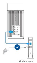
4 Check the modem LED lights to ensure the connection is active.
