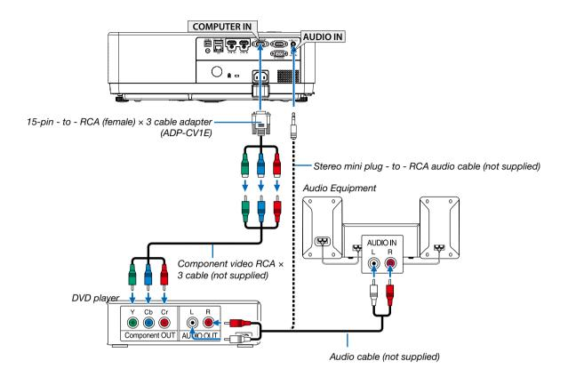
• Select the source name for its appropriate input terminal after turning on the projector.
