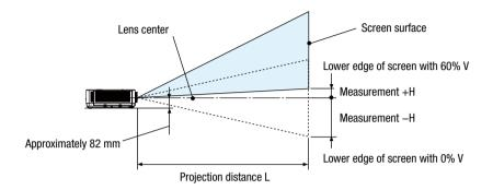
(NOTE) Height from lens center to lower edge of screen (with tilt feet screwed in)
