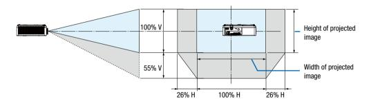
(Example) When using to project on a 150" screen
