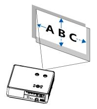
Rotate 1 dial, then you can move upward and downward the image with a distance up to +55% (PE506WL) and 60% (PE506UL) between the upper and lower range of the image.
