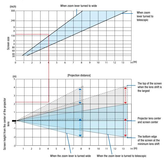
\* The figures indicated for "height of screen from projector lens center" on the projection distance table are for a lens shift of 55% V.
