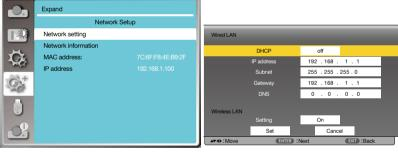
Press the ▲▼ button to set DHCP "Off", then press the ENTER button to enter an IP address, then press ▼ button to enter Subnet, Gateway and DNS manually. And press the ENTER button to confirm.
