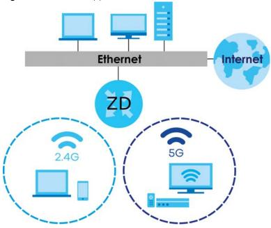
The Zyxel Device is a wireless Access Point (AP) for IEEE 802.11b/g/n/a/ac/ax wireless clients, such as notebook computers, iPads, smartphones, and so on. It allows them to connect to the Internet without having to rely on inconvenient Ethernet cables.
