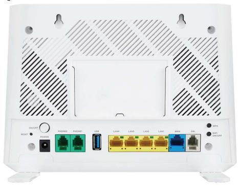
**Figure 15** DX5301-B2 / DX5301-B3 Back Panel
