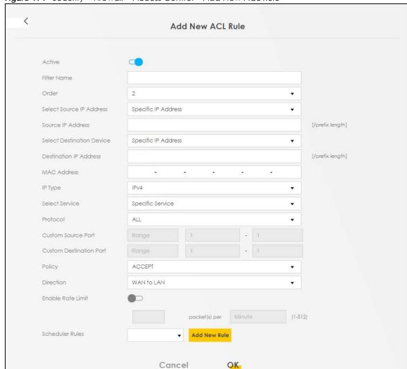
Figure 174 Security > Firewall > Access Control > Add New ACL Rule
