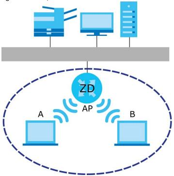
The WiFi network is the part in the blue circle. In this WiFi network, devices **A** and **B** use the access point (**AP**) to interact with the other devices (such as the printer) or with the Internet. Your Zyxel Device is the AP.
