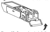
Figure 25 Transceiver Installation Example
