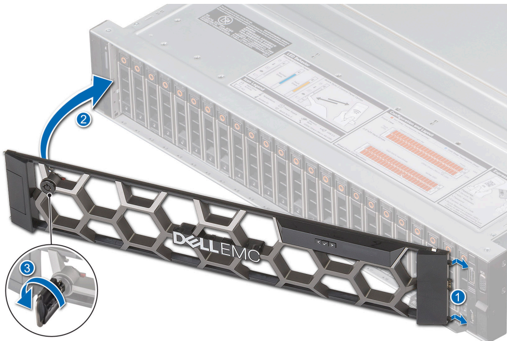
Figure 18. Installing the front bezel with the LCD panel
